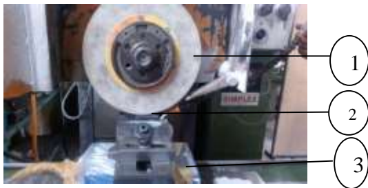
1-Grinding Wheel, 2-Workpiece, 3-Dynamometer (a) Grinding machine setup
